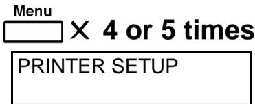
2. Press the **Menu** key four or five times (when an optional hard disk drive is installed).
