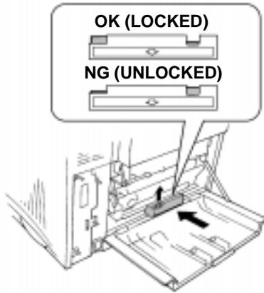
21. Make sure that the **fusing unit lock release button** is pushed up as shown.
