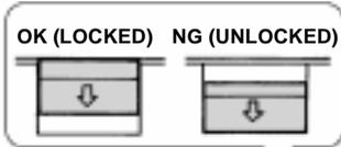
11. Make sure that the button of the **lock release lever** is pushed up as shown.
